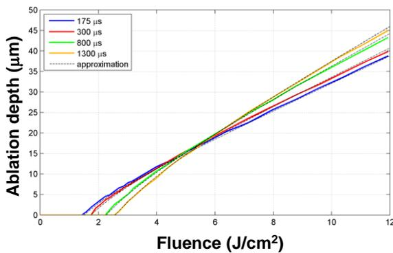
Fig. 9: Dependence of skin ablation depth on laser pulse fluence and pulse duration, as calculated from the MEC micro-explosions computer model.
