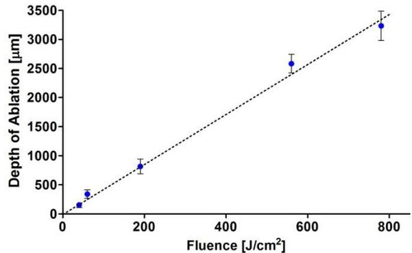
Fig. 14: Dependence of ablation depth on micro beam fluence for the F22 scanning fractionated handpiece, as obtained from histological results. The ablation depth ( $D$ ) depends linearly on the maximal pulse fluence within a micro beam as  $D = K \times (F - F_{\text{thr}})$  where  $K = (4.3 \pm 0.2) \mu\text{m cm}^2/\text{J}$ .
