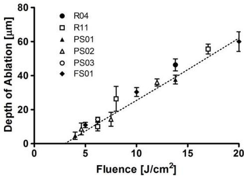
Fig. 12: Dependence of ablation depth on laser pulse fluence and handpiece type, as measured with the laser triangulation method). The ablative depths follow the same linear dependence of laser full beam or micro beam fluence, independently of the handpiece type. The ablation depth ( $D$ ) depends linearly on the pulse fluence ( $F$ ) as  $D = K \times (F - F_{\text{thr}})$  where  $K = (3.7 \pm 0.4) \mu\text{m cm}^2/\text{J}$ .
