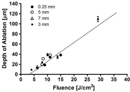
Fig. 11: Dependence of ablation depth on laser pulse fluence and spot size, as measured with the laser triangulation method using full beam R04 handpiece and fractionated FS01 handpiece, 300  $\mu$ s pulse duration). The ablation depth ( $D$ ) depends linearly on the pulse fluence ( $F$ ) as  $D = K \times F$  where  $K = (3.8 \pm 0.3) \mu\text{m cm}^2/\text{J}$ .
