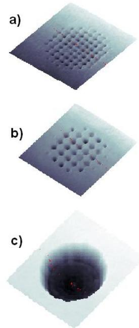
Fig. 8: Triangulation images of the ablated holes following a treatment with: a) stamping patterned handpiece PS01, position 1.7mm overall spot size; b) stamping patterned handpiece PS01, position 3.7mm overall spot size; c) full beam handpiece R04, 7 mm spot size.
