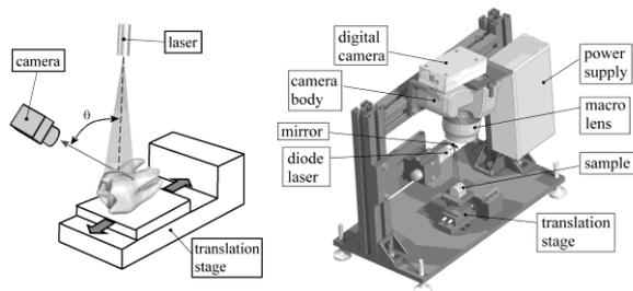
Fig. 6: Schematic showing operation of profilometer, and general assembly of the equipment.
