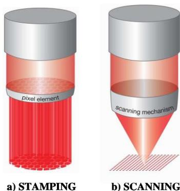
Fig. 3: Two types of fractionated handpiece technologies.
