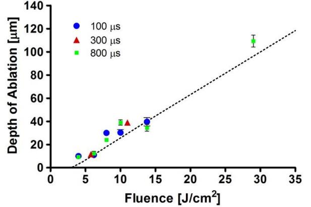
Fig. 10: Dependence of human skin ablation depth on laser pulse fluence and pulse duration, as measured with the laser triangulation method (R04 handpiece, 3 mm spot size). The ablation depth ( $D$ ) depends linearly on the pulse fluence ( $F$ ) as  $D = K \times F$  where  $K = (3.7 \pm 0.3) \mu\text{m cm}^2/\text{J}$ .
