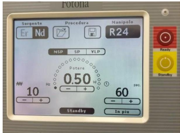
Figure 5: Fotona AT-Fidelis laser's working parameters
