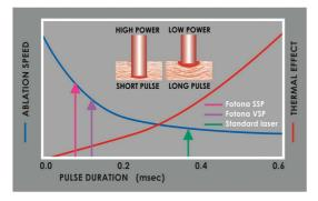
Fig.6: Keeping the pulse energy constant, the ablation efficiency increases, and the thermal effects decrease towards shorter pulse durations. Due to the long cross-relaxation time of the  $Cr^{3+}$  ion, the Er,Cr:YSGG cannot be operated bellow approximately 500  $\mu$ s.
