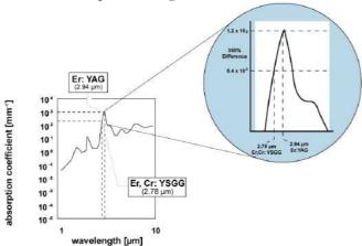
Fig.1: The Er:YAG (2.94  $\mu m$ ) laser has the highest absorption in water and hydroxiapatite. An alterantive laser that emits in the 3  $\mu m$  region is the Er,Cr:YSGG (2.78  $\mu m$ ) laser, however this laser has a 300% lower absorption and is thus less suitable for laser drilling.
