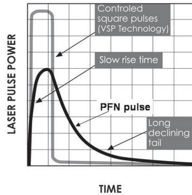
Fig. 20. Comparisons between PFN and VSP shaped pulses.
