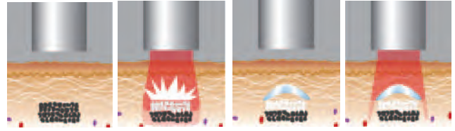
Fig. 23: Whitening results in an optical shield that prevents subsequent pulses from reaching the remaining underlying pigments.
