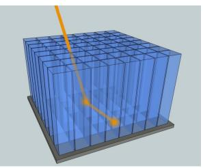
Fig. 1: Inelastic scattering of a gamma photon, followed by photoelectric absorption, serves as a precise relative temporal marker for any pair of 64 readout channels in a TOF PET detection block.
