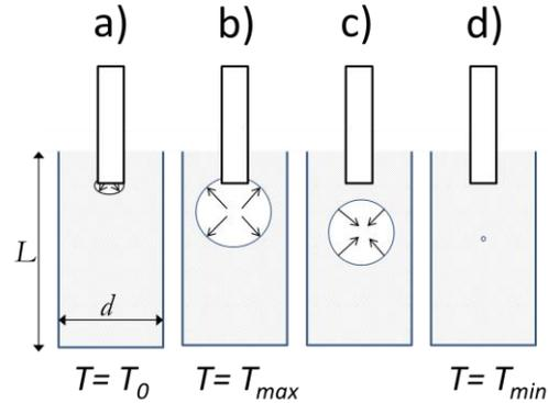
Fig. 1: Cavitation bubble oscillation sequence following the emission of a single Er:YAG laser pulse. A vapor bubble starts to expand when a laser pulse is emitted at  $T=T_0$  (a) until the bubble reaches its maximum size at  $T=T_{max}$  (b), after which the bubble starts to collapse (c) until it reaches its minimal size at  $T=T_{min}$  (d) and rebounds. In narrow root-canal like reservoirs, the bubble collapse is too slow to result in the emission of shock waves.
