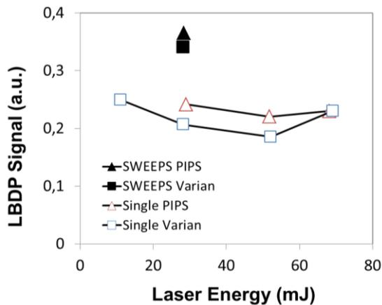
Fig. 7: Measured dependence of the pressure amplitude (LBDP signal) following the collapse of the initial bubble on the individual laser pulse energy for a flat (Varian) and conical (PIPS) tip under single pulse and SWEEPS conditions, for a 6 mm diameter canal.
