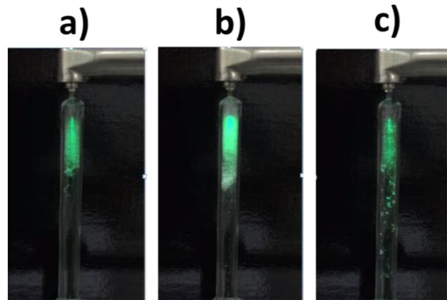
Fig. 8: Images of cavitation bubbles during an Auto SWEEPS cycle as the temporal separation between the SWEEPS laser pulse pair is being swept from a) long separations ( $T_p > T_{opt}$ ) to c) short separations ( $T_p < T_{opt}$ ). Fig 7 (b) shows formation of cavitation bubbles when the pulse separation approached the optimal separation,  $T_p \approx T_{opt}$ .
