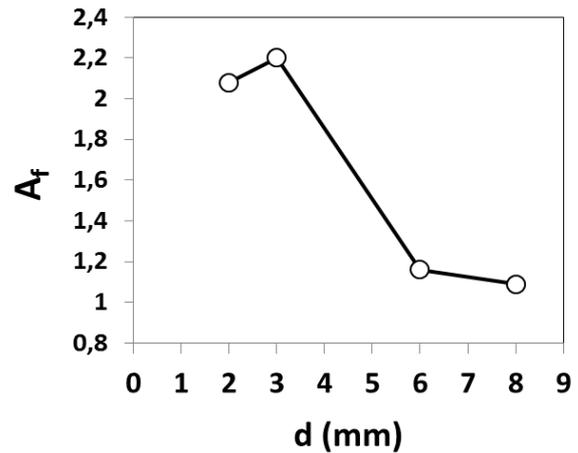
Fig. 6: The factor of increase in the LBDP amplitude of pressure waves generated by the SWEEPS technique, in comparison to the pressure waves generated by the standard PIPS technique. The amplification is strongest in narrow canals where the acceleration of the bubble collapse is largest in comparison to the speed of collapse in an infinite reservoir. The line is a visual aid only.
