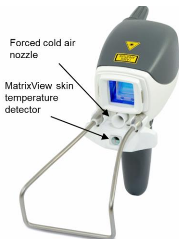
Fig. 5: The L- Runner: an advanced Nd:YAG laser scanner with MatrixView camera sensor for on-line skin temperature measurement.
